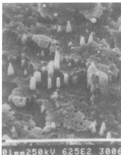
Figure 6. SEM fracture surface of an extruded strand of PA1/LDPE1/SEBS-g-DEM 20/80/5 blend.
